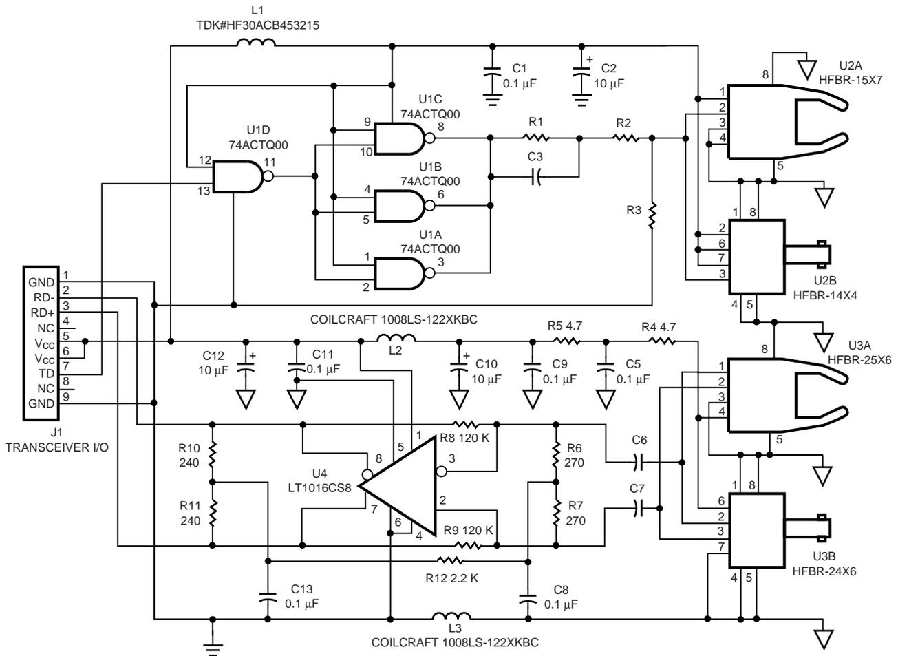
Figure 11. Transceiver Circuit
